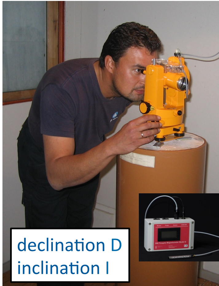
fluxgate theodolite (DI-flux)
